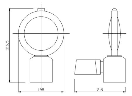
Weight (excluding battery) Standard zinc carbon battery DAAB25 air alkaline battery DAAB50 air alkaline battery 642g 540g (each) 640g (each) 740g (each)
